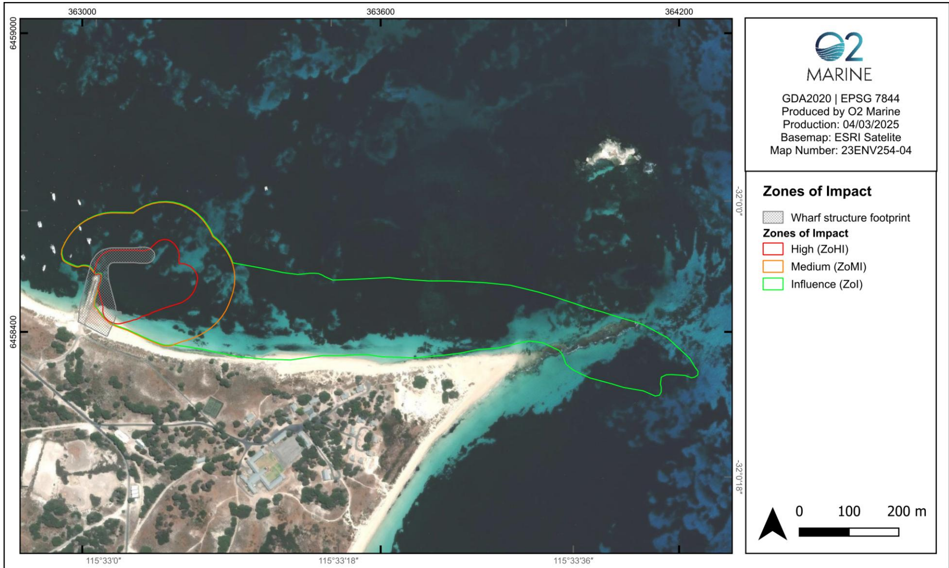
Figure 6: Wharf structure and dredging zones of impact (Source: Baird (2024))
