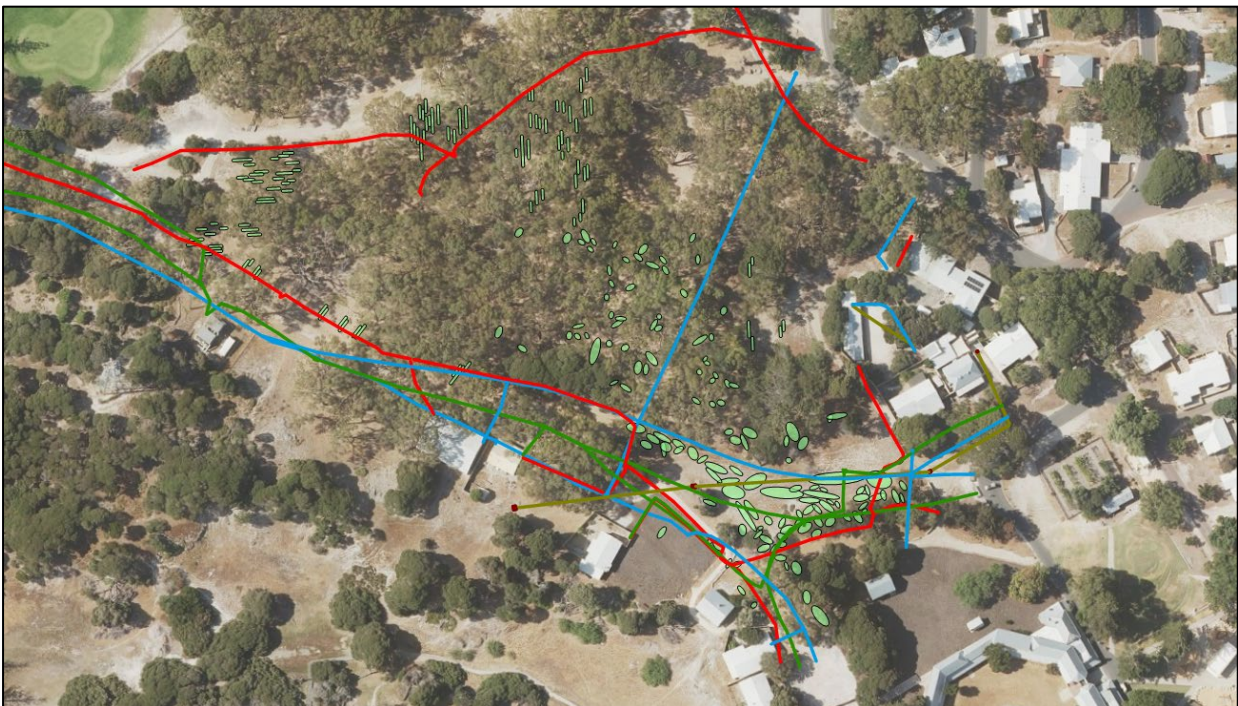
Figure 4: Identified underground utilities across the WABG, overlaid with the 1991 and 2004 anomaly shape files (green).
